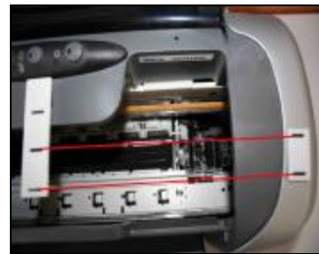
Rip the label on the balance arm
